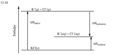
Lattice energy values are always positive as energy is required to separate the ions from each other. Hydration energy values are always negative as energy is released when intermolecular forces between ions and water form. Since the heat of solution for KCl is endothermic, the lattice energy must be greater than the hydration energy for an overall input of energy.
