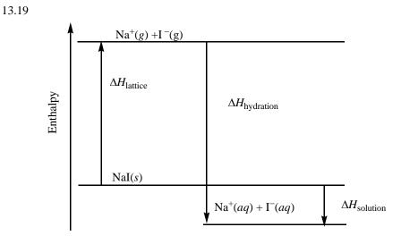
Lattice energy values are always positive as energy is required to separate the ions from each other. Hydration energy values are always negative as energy is released when intermolecular forces between ions and water form. Since the heat of solution for NaI is exothermic, the negative hydration energy must be greater than the positive lattice energy.
